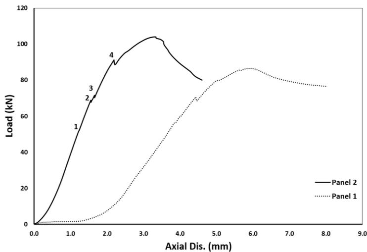
Fig. 4 Load vs axial displacements for panels with  $R=400\text{mm}$
