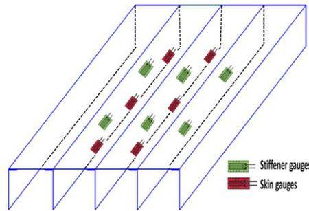
Fig. 2 Strain gauge positions map
