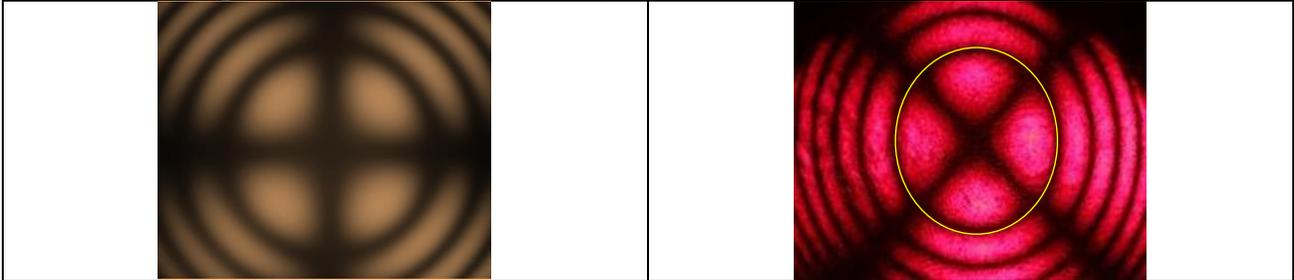
Figure 3 Fringe pattern acquired by diffused light polariscope in conoscopic modality. Unstressed Uniaxial crystal on the left, acquired by diffused light polariscope. Compressed Uniaxial crystal on the right, acquired by laser conoscopic technique; the yellow line is the fitted CL into the first fringe order by which the stress state is evaluated.
