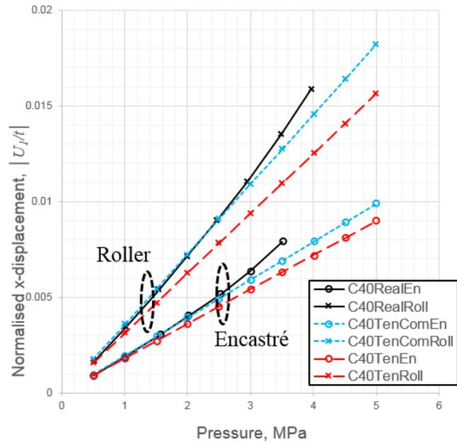
Figure 2 Displacement around the plate edges normalised to the plate thickness
