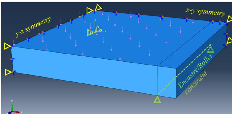
Figure 1 Quarter model of plate with distributed pressure loading.
