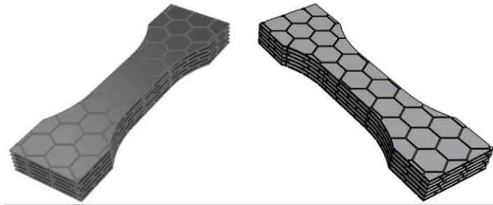
Fig. 2. Design schematic showing (left) the distribution of soft matrix material with the complementary hard counterpart made of platelets (right) from the generative design algorithm.
