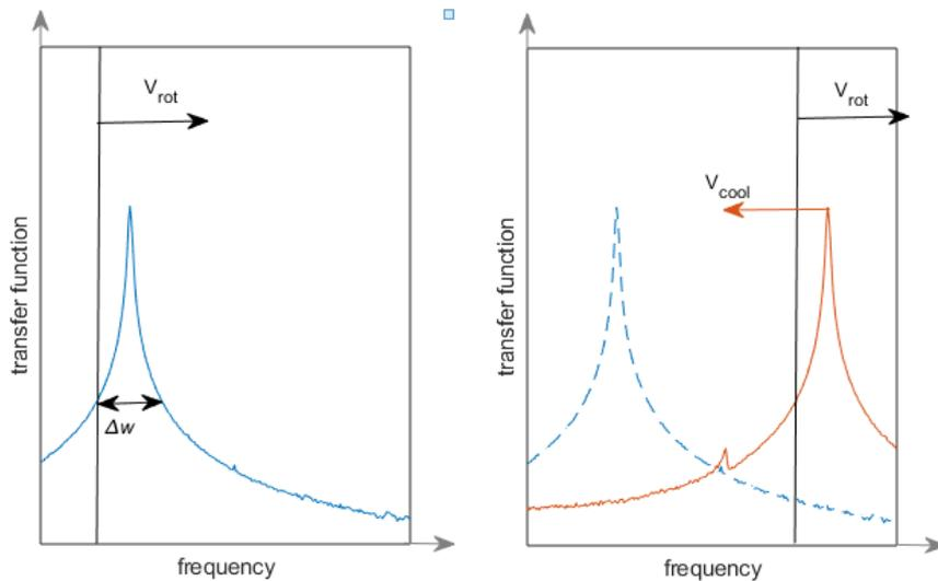
Figure 4 When rotor speed of a aeroengine gradually increases or decrease, the resonant time can be reduced by manipulating the shape memory alloy heating.
