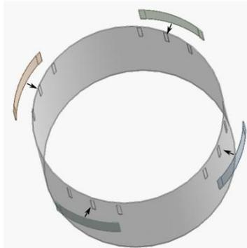
Figure 1 Titanium alloy cylinder attached with four shape memory alloy actuators plates.
