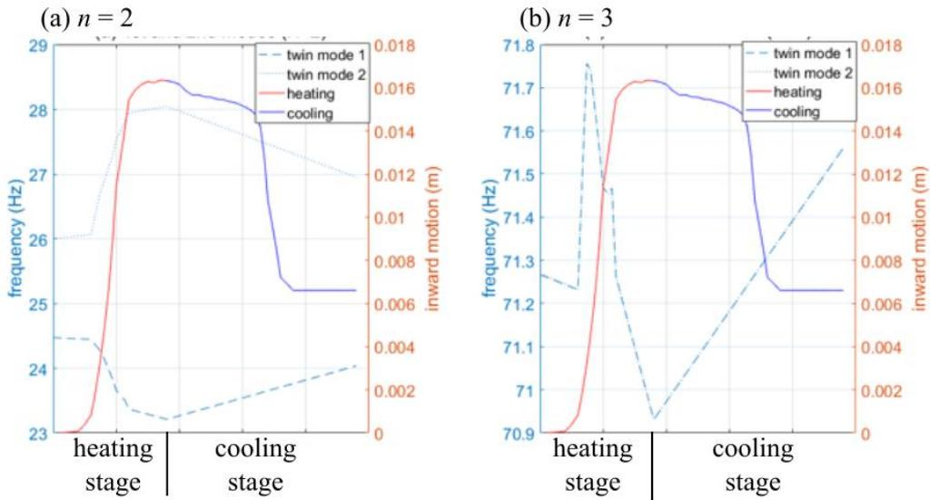
Figure 2 Both graphs shows the static deflections (solid curves) and natural frequencies (dotted and dashed lines) against varied temperature. The dotted and dashed line represented a pair of twin modes in cylindrical structures. The left graph shows the information of a resonant mode with circumferential node of  $n = 2$ , while the right graph shows the mode with  $n = 3$ .
