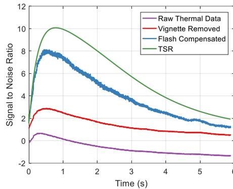
Figure 1: Processing PT inspection data [4]
