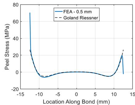
Figure 2: Transverse normal stresses along bond line
