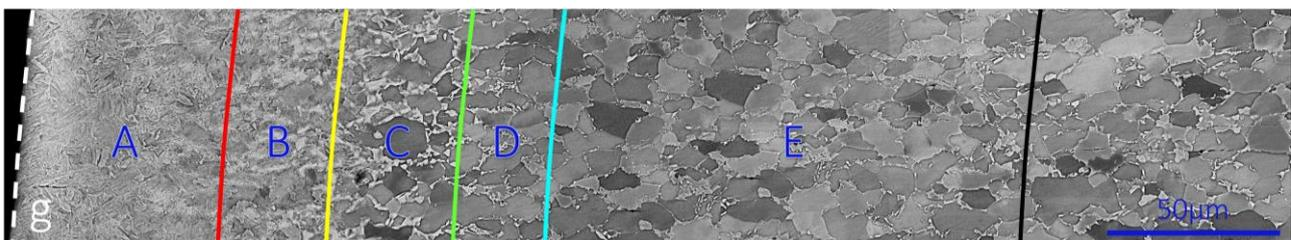
**Figure 1:** Secondary electron (SE) image of the different microstructures in the heat-affected zone of a laser-cut specimen (the white dashed marks the cutting edge)
