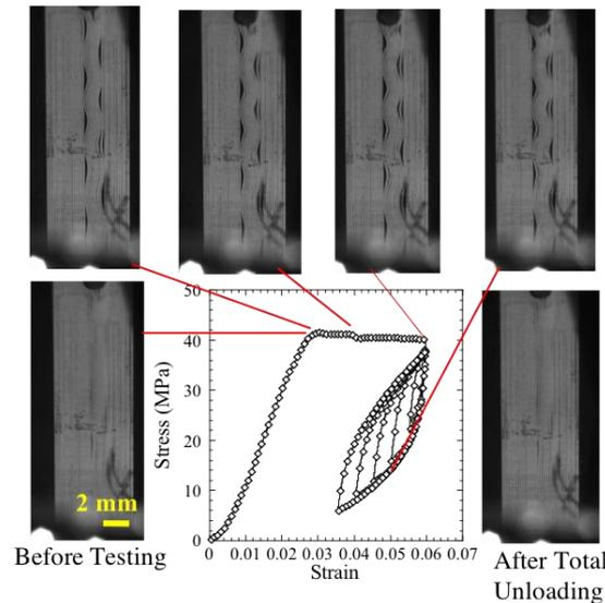
Fig 1. Image of a typical indenter loading cycle on plastic layers, highlighting reversible ripple formation.
