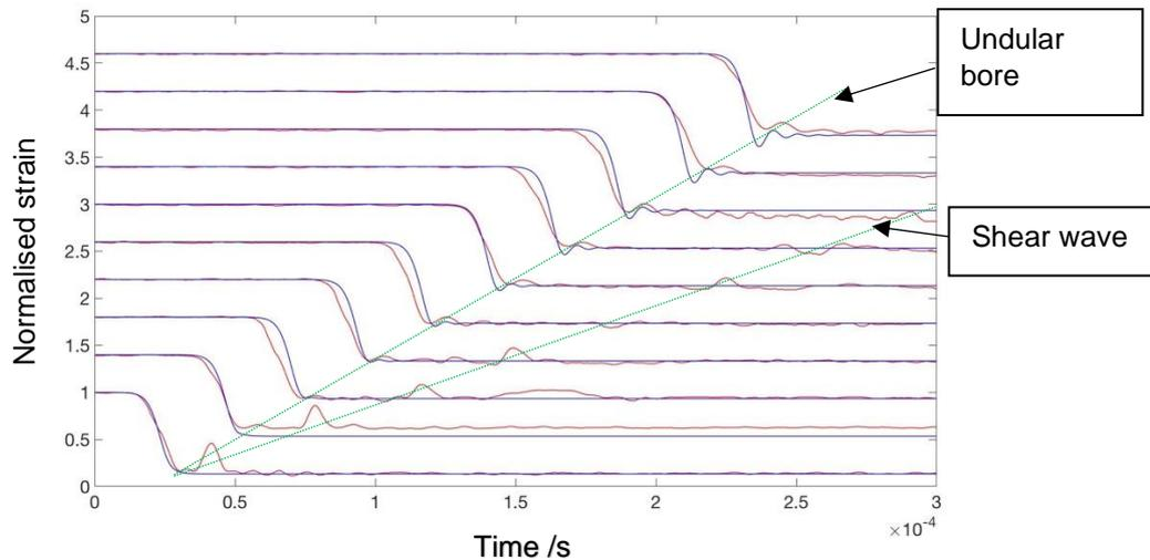
**Fig 3.** Experimental (red) and model (blue) strain profiles recorded every 50 mm from the notch. Each profile has been normalised by the strain present in the bar at the time of fracture. A vertical offset is given between each plot for clarity. The two observed waves are tracked by the green (dashed) lines.
