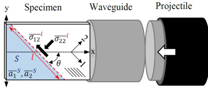
Figure 1. Schematic showing the main components of the IBI test with an off-axis composite specimen.
