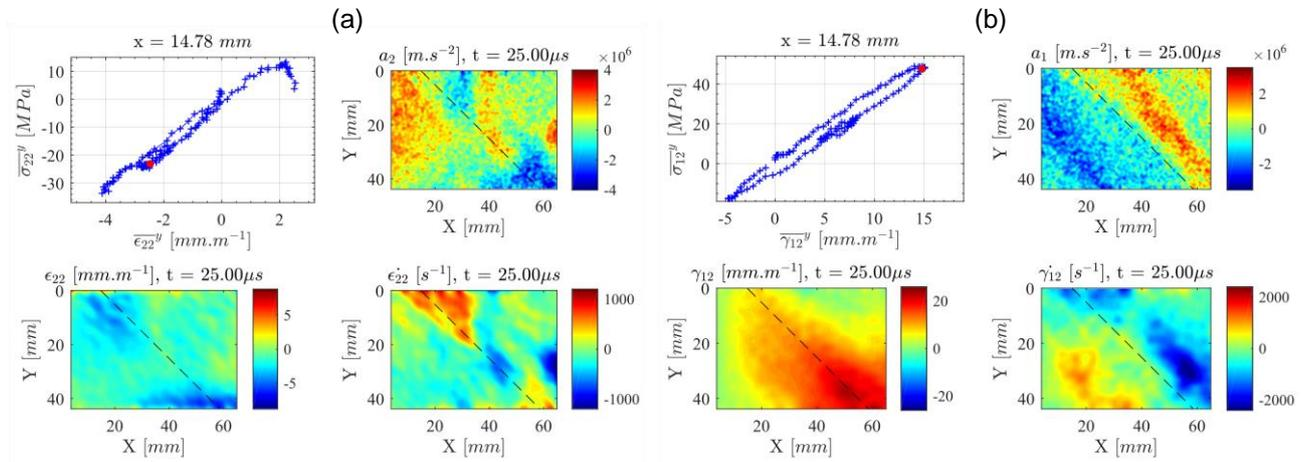
Figure 2. Kinematic fields and stress-strain response for the (a) transverse component and (b) shear component.
