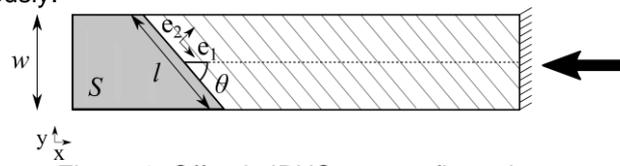
Figure 1: Off-axis IBUS test configuration
