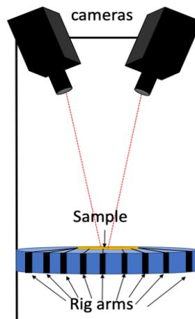
Figure 2 – Radial Stretch Tester with DIC
