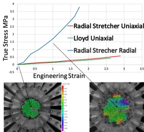
**Figure 4 – True stress vs engineering strain data for three tests of Versaflex™ CL200X**
