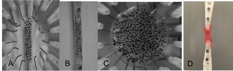
**Figure 3 - uniaxial with hooks (a), uniaxial with velcro clamps (b), and (c) radial with hooks (all with speckle for DIC), (d) sheep tissue**
