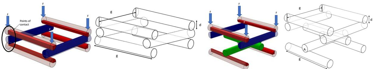
Figure 1. Unit volume elements of aligned (left) and offset (right) fused filament scaffolds.
