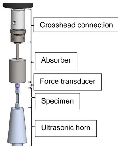
Fig 1. Test apparatus with absorber
