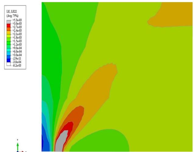
Fig. 04 Linear Elastic Strain  $\epsilon_{22}$  shown for  $a/W=0.1, b=5\text{mm}$
