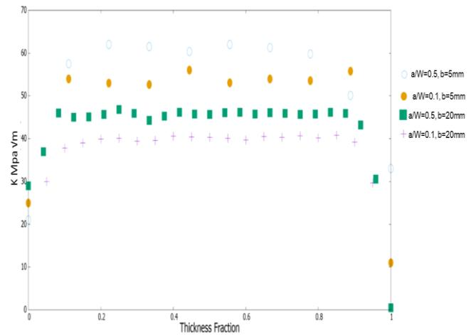
Fig. 03 Graph of  $K$  values through thickness from FE
