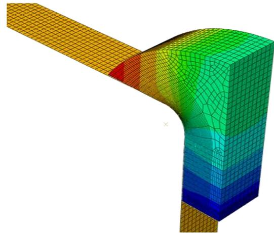
Fig. 02 Image of geometry of simulation .showing FE mesh
