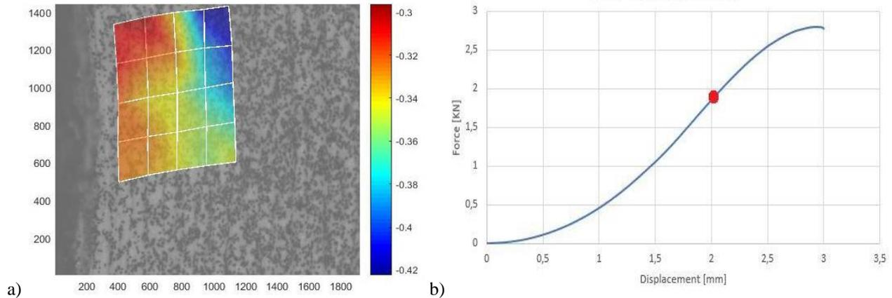
Figure 2: a) strain distribution, b) load-displacement curve
