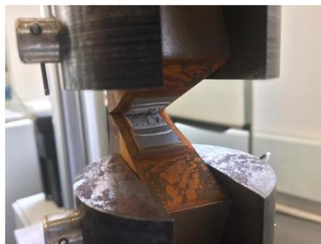
Fig 1 – a) welded plate with compact tension samples cut out using electro discharge machining from the parent and the weld b) example of the fracture surface of sample made of parent material
