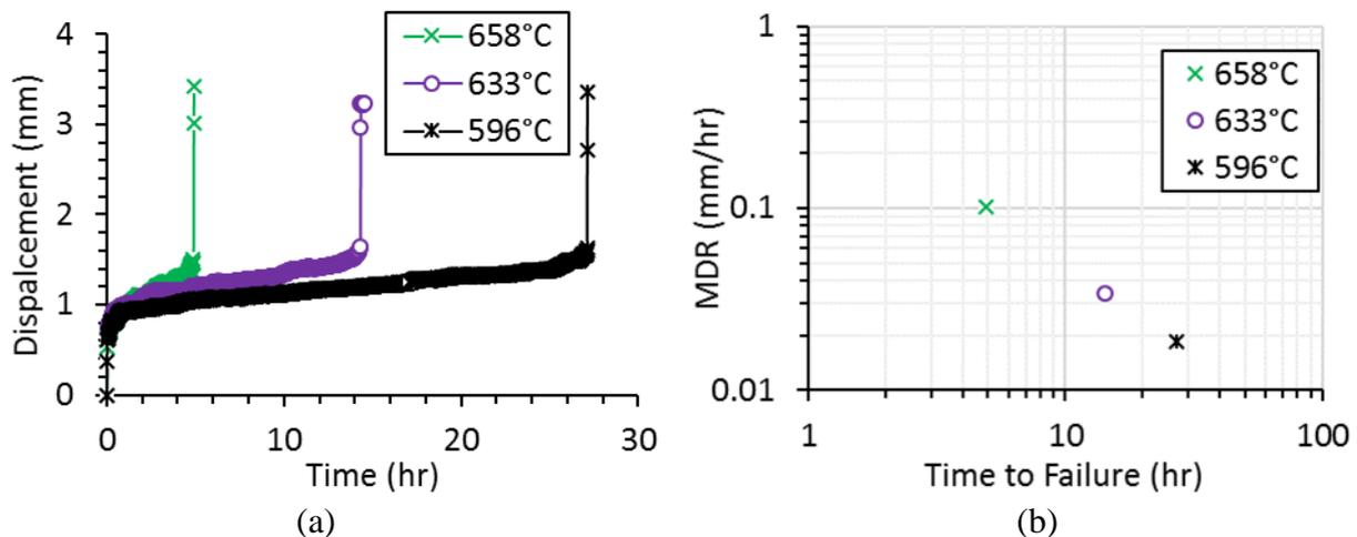
Figure 2. a) Displacement versus time curves and b) minimum displacement rate versus time to failure for P91 tested at 658, 632 and 595°C.
