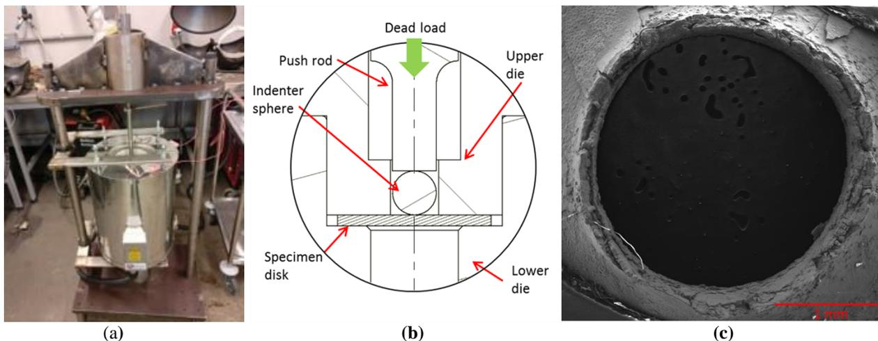
Figure 1. a) NUI Galway SPC test apparatus, b) Section view schematic of indenter, die and specimen inside of furnace and c) SEM image of ring fracture surface of sample tested at 600°C
