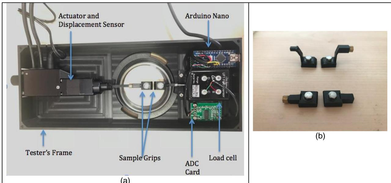
**Fig 1: Images of (a) Internal setup of the micromechanical tester (b) Example of 2 different types of grips L-shaped grips (top) and straight grips (bottom).**
