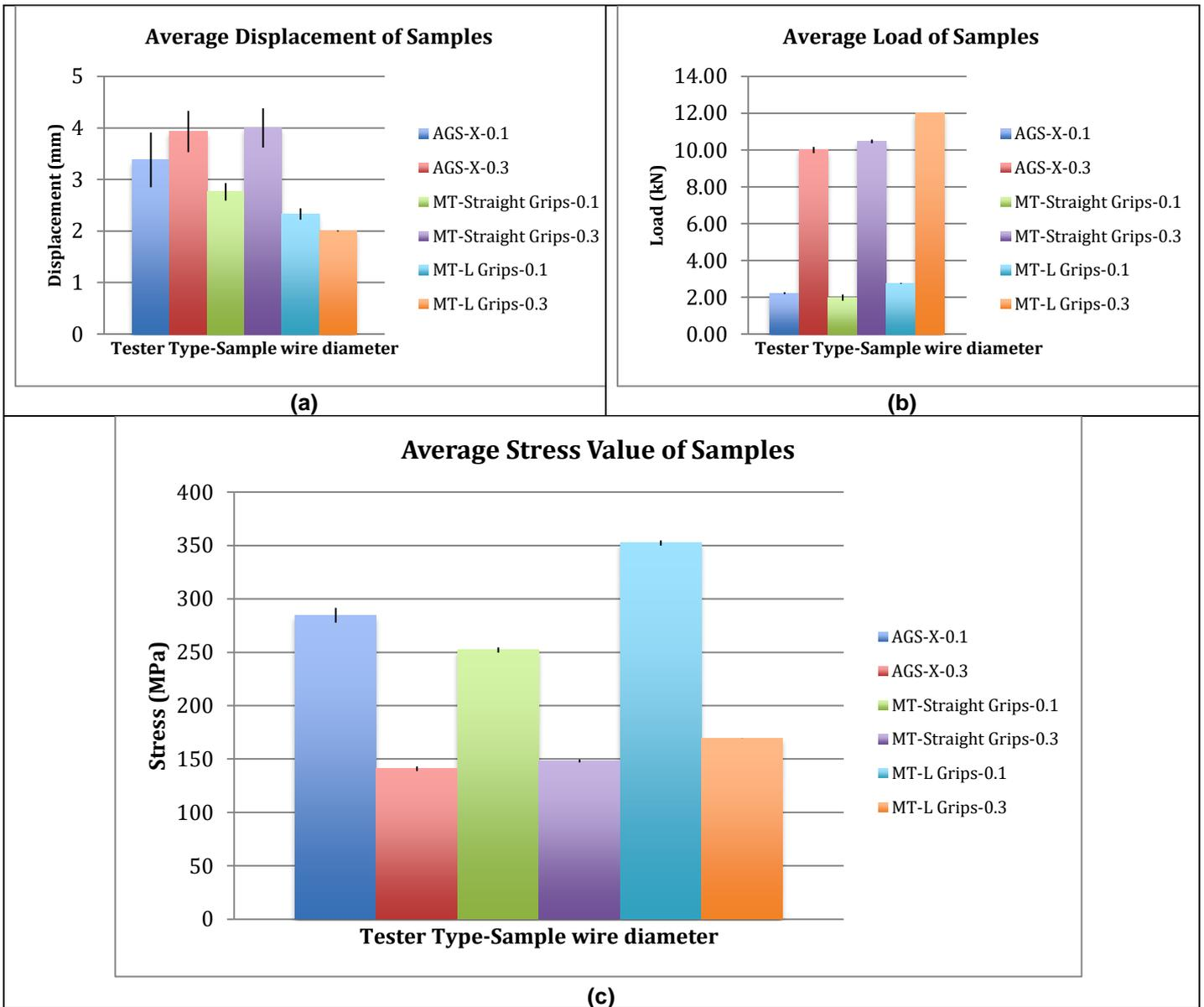
**Figure 2: Graphical results on copper wire tensile tests from Shimadzu model AGS-X tester and prototyped micromechanical tester denoted by MT with different straight and L-shaped grips. (a) Shows the average displacement (b) average load at which the wire fractures and (c) average maximum stress value measured for 0.1mm and 0.3 mm specimen on the different testers and different grips.**
