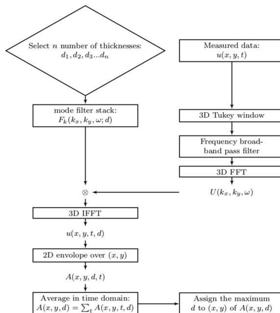
Figure 1: Mode filtering algorithm
