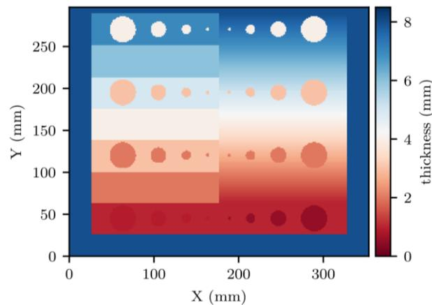
**Figure 2:** Phantom true thickness map
