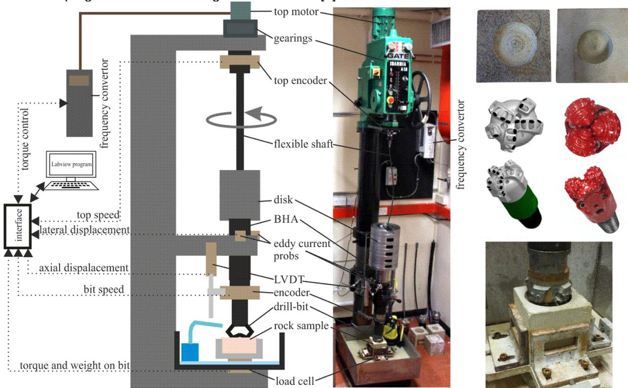
**Figure 1:** (left) Schematic diagram of the experimental setup, (middle) photograph of the experimental rig and (right) examples of rock samples and drill-bits used in the setup. Main components of the system are: sensors (top and bottom encoders, eddy current probes, LVDT and 4-component load cell), electric motor, flexible or rigid shafts, disks, the BHA, drill-bit and rock samples.
