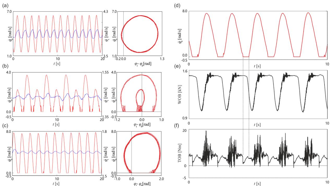
**Figure 2** Examples of experimental time histories and phase portraits of (a) torsional vibration for WOB of 1.13 kN, (b and c) stick-slip oscillations for WOB of 1.95 and 1.4 kN respectively. Experimental time histories of WOB (e) and TOB (f) during stick-slip oscillations as shown in panel (d).
