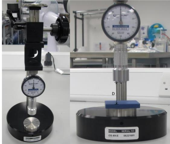
**Figure 1 – Left: Checkline® AD-100 Precision Shore Durometer and RX-OS-4H-E test stand, Right: Distance from test piece to presser foot**
