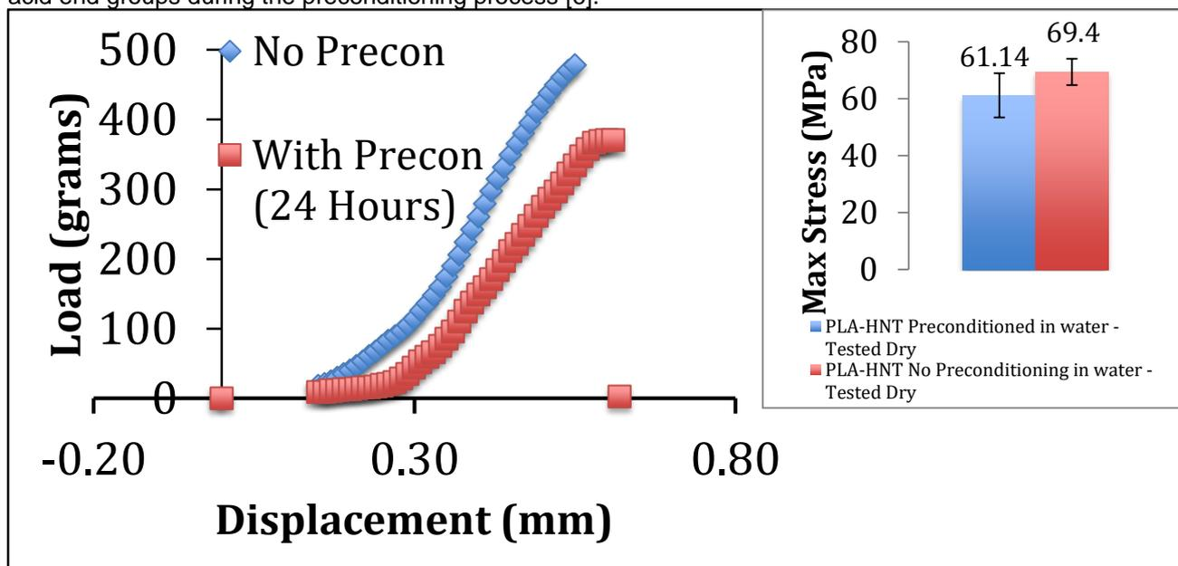
Figure 2: Load vs Displacement graph showing the difference in maximum load at which samples with preconditioning and without preconditioning fractures. Corresponding bar chart illustrating maximum stress of PLA-HNT polymer blends in the different test conditions.
