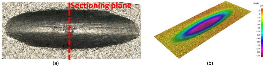
Figure 1: (a) Blunt dent on a Nickel alloy; (b) 3D profile of a dent by an Alicona InfiniteFocus microscope.
