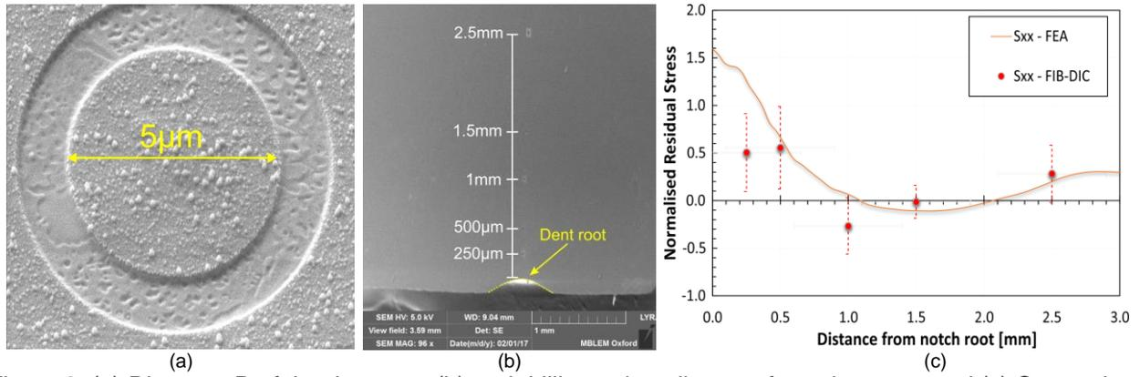
Figure 3: (a) Diameter  $D$  of the ring core; (b) and drilling points distance from dent root; and (c) Comparison between residual stress  $\sigma_{xx}$  predicted by the FE model and measured by FIB-DIC.
