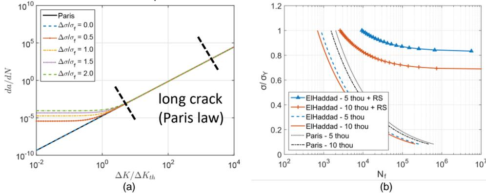
Figure 4: (a) Crack growth law with El Haddad modification; (b) Predicted fatigue life for 5 and 10 thou dent depths with and without residual stresses.
