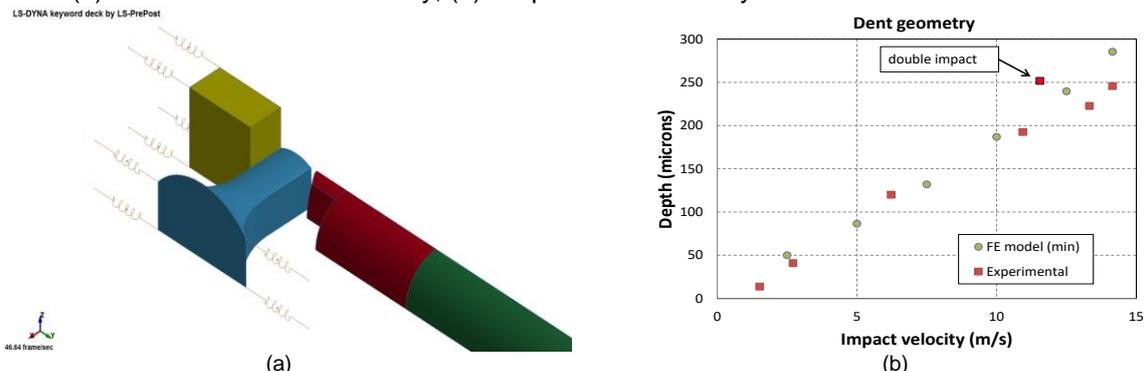
Figure 2: (a) FE model used in LS-Dyna; (b) Experimental and FE dent depth as a function of impact speed.
