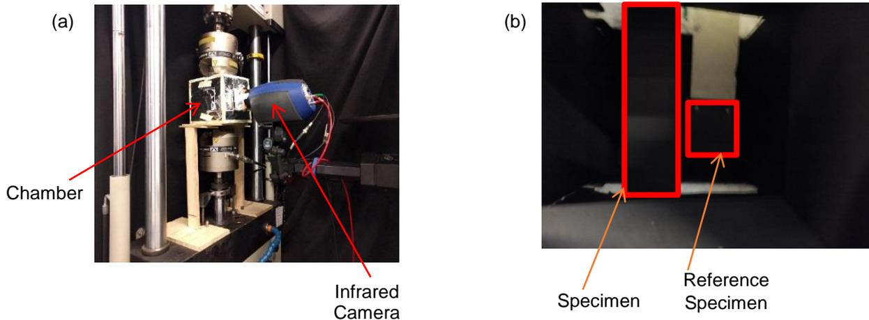
Figure 1(a) Setup of the actual experiment (b) specimen and reference specimen
