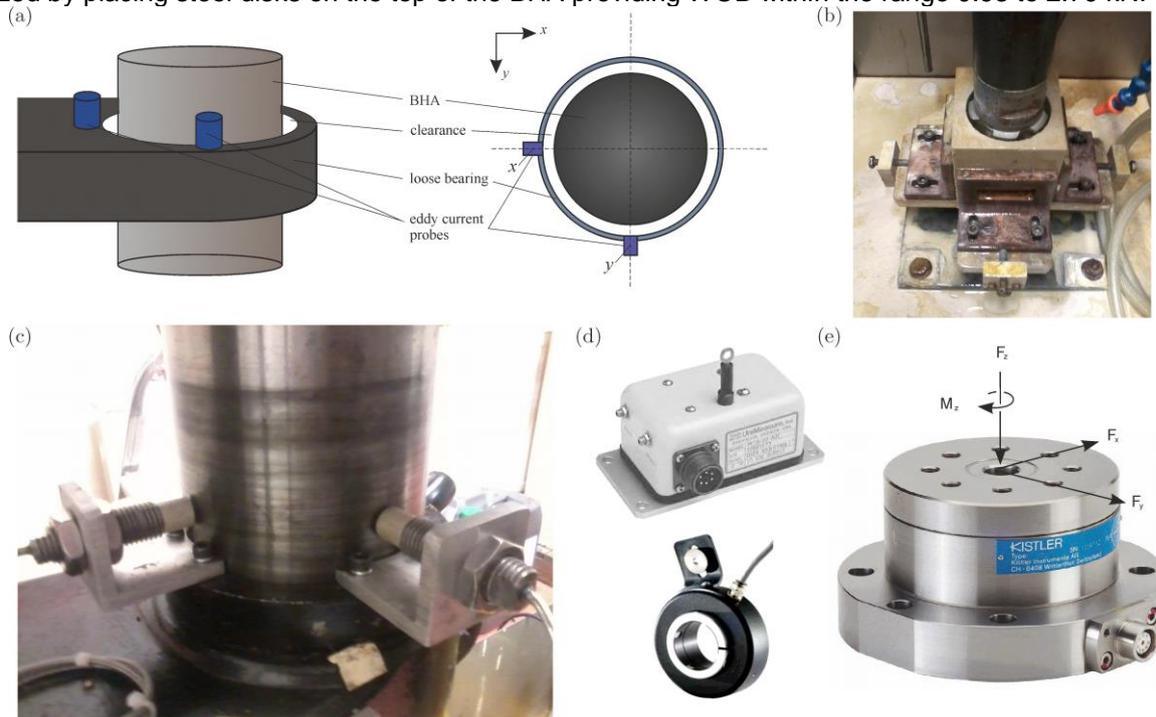
Figure 1 (a) Schematic diagram and photograph of the experimental setup. Main components of the system are: electric motor, flexible or rigid shafts, disks, the BHA, drill-bit and rock samples. (b) Drill-bit rock interface and the BHA with position of the eddy current probes, (c) 4-component load cell (d) top and bottom encoders and LVDT.
