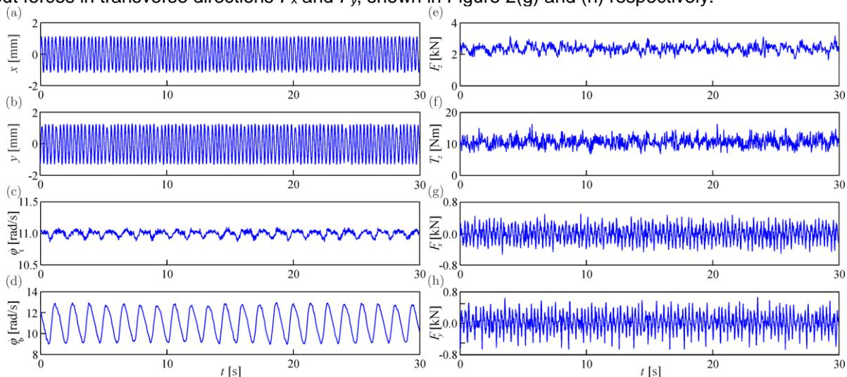
Figure 2 A sample of the recorded experimental time histories for configuration with 20 disks; (a) and (b) displacement of the BHA in the  $x$  and  $y$  direction respectively, (c) and (d) top and bottom speed, (e)  $F_z$ , (f)  $T_z$ , (g) and (h) transverse forces on  $x$  and  $y$  direction acting on the drill-bit.
