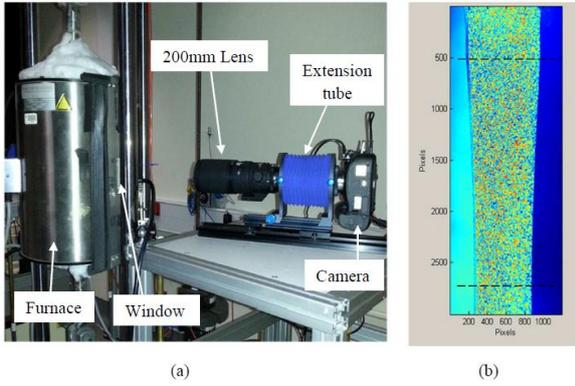
Figure 2. (a) Experimental set-up for DIC monitored creep test of the waisted specimen (b) the specimen as viewed through the furnace window.
