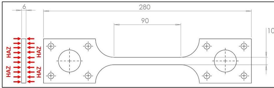
**Figure 2:** Tensile specimen dimensions (mm)
