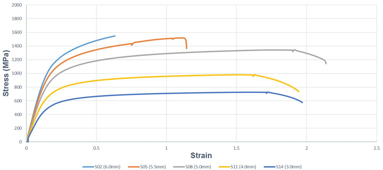
**Figure 3:** Stress/Strain curves from the ground tensile specimens.
