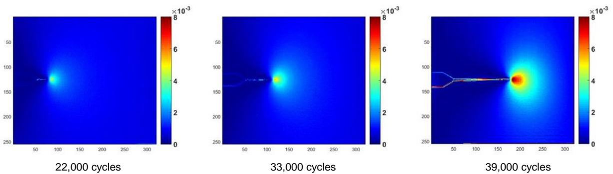
Figure 2. Thermoelastic response evolution ( $\Delta T/T$ ) from TSA.
