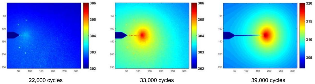
Figure 1. Specimen temperature evolution from IRT.
