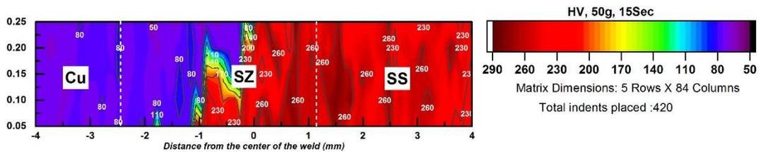
**Fig. 2 Microhardness 2D-contour map of Cu-SS FSW joint over the region shown in Fig. 1**
