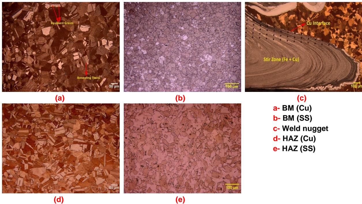
**Fig. 3 Microstructures at different zones of the friction stir welded Cu-SS Joint**
