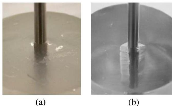
Figure 1: Image of needle inserted into gel phantom which a) does not exhibit tearing b) tears [4].
