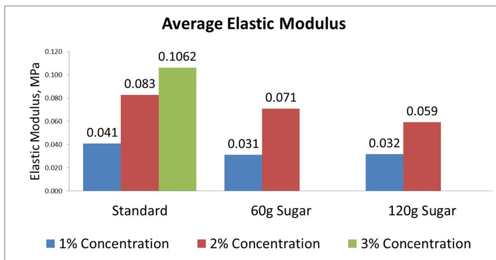
Figure 2: Image depicting the calculated elastic modulus for various concentrations of carrageenan
