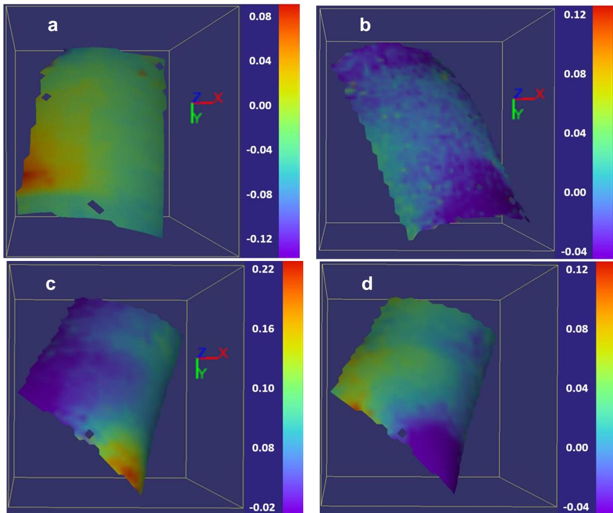
**Figure 2.** Full field tangential strain distributions at the maximum pressure level of 81 kPa (11.75 psi). Shear strain (a) and Y-strain (b) on the white critical layer of the full coverage garment. Y-strain (c) and X-strain (d) on the green protective layer of the skeletal garment.
