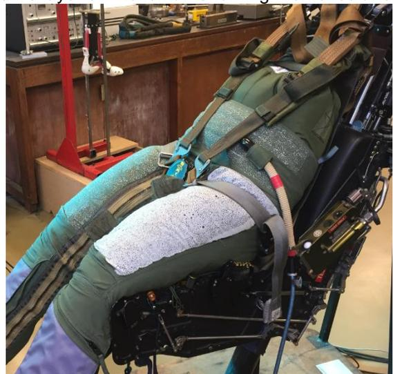
**Figure 1. Full Coverage Garment fitted to ATD secured to a Martin Baker Type 12H Mk2 ejection seat**
