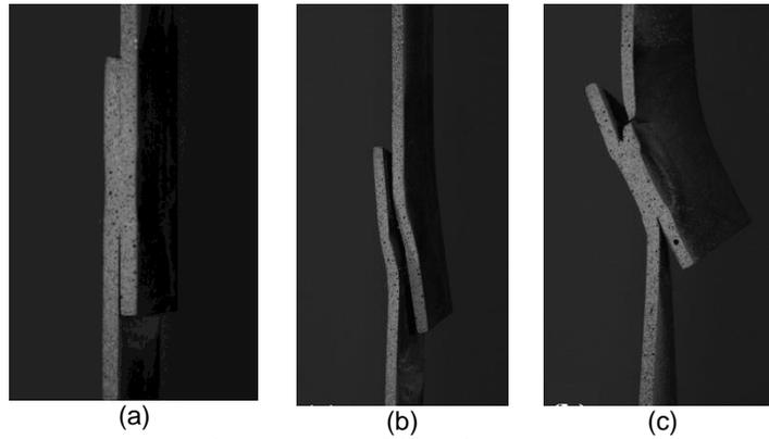
Figure (1) (a) speckle patten produced on 1 mm thick HX340LAD samples to determine the failure mode on the spot welds due to uniaxial tensile loading, showing examples of (b) an interfacial failure for small weld size and (c) a pull-out failure for a large weld size.
