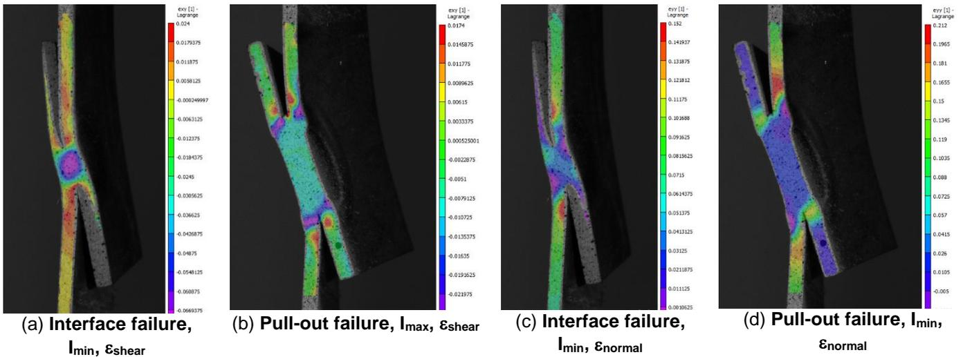
Figure (3) (a, b) shear strain( $e_{xy}$ ) and (c,d) normal strain ( $e_{yy}$ ) distributions for the HX340LAD samples experiencing (a, c at minimum current) interfacial and (b,d at maximum ) pull-out failure mode. The loading direction in all images are vertical and the  $e_{yy}$  strain corresponds to the strain in the loading direction
