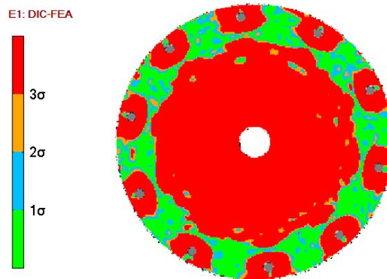
Figure 2. E1: DIC - FEA validation map. Difference is the Yield Stress (450 MPa (DIC) vs 500 MPa (FEA)). As a result deformations for DIC are larger at the same force. Red areas indicate errors that fall beyond the noise floor.
