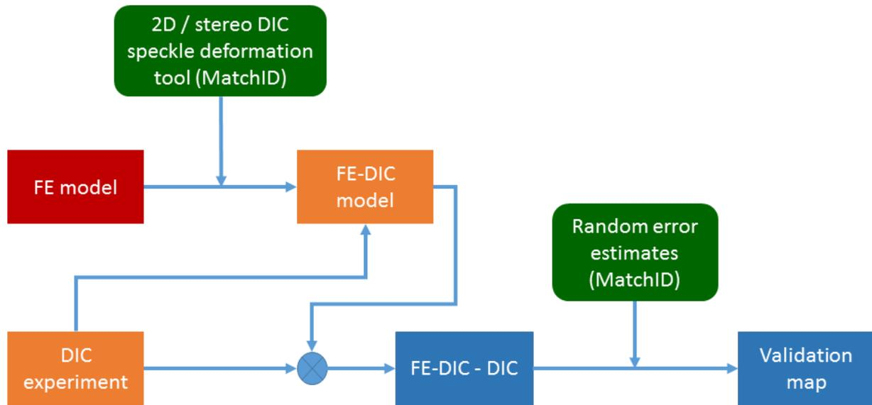
Figure 1: Flowchart of the proposed FE model validation process
