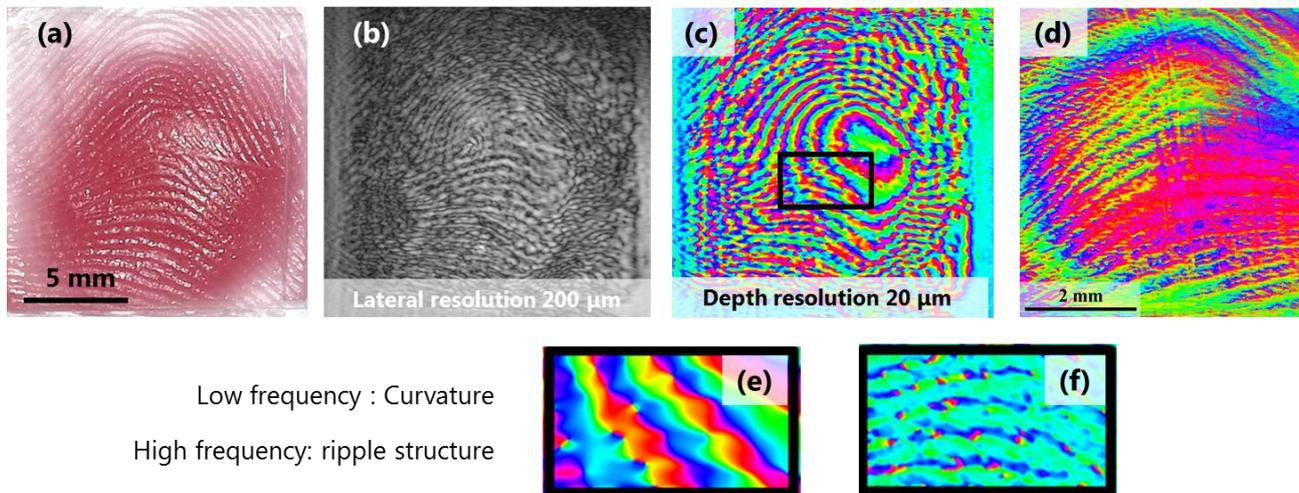
**Figure 2:** The object (a), the reconstructed intensity (b) and reconstructed phase map (c). The phase map contains information on both the overall curvature (e) and ripple structure (f). For comparison, a fringe projection measurement through the plate is given in (d).
