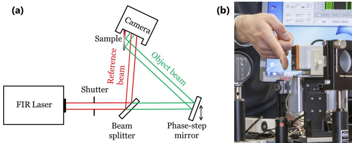
**Figure 1:** Schematics of the THz off-axis digital holography set-up in reflection (a) and a close up of an object behind a plate (b).
