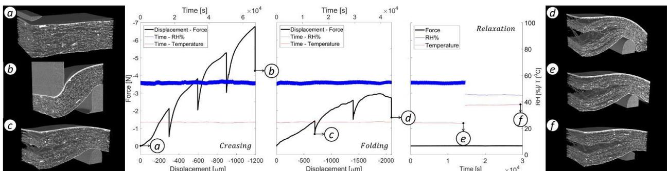
**Figure 2:** High-resolution 3D CT characterization of hygro-thermo-mechanical response of cardboard under creasing and folding.[1]
