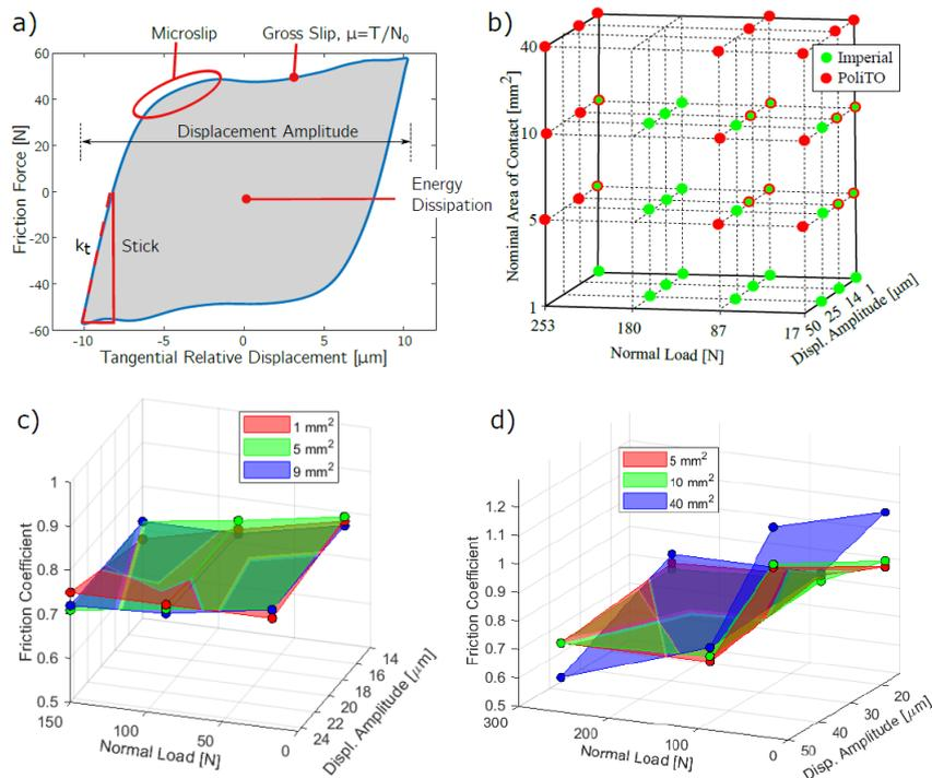
Fig. 1. a) Typical hysteresis loop ( $\mu$  is the friction coefficient,  $k_t$  is the tangential contact stiffness,  $T$  is the friction force during gross slip and  $N_0$  is the normal load); b) round robin test matrix; c) steady state values of  $\mu$  for the Imperial friction rig; d) steady state values of  $\mu$  for the PoliTO friction rig.
