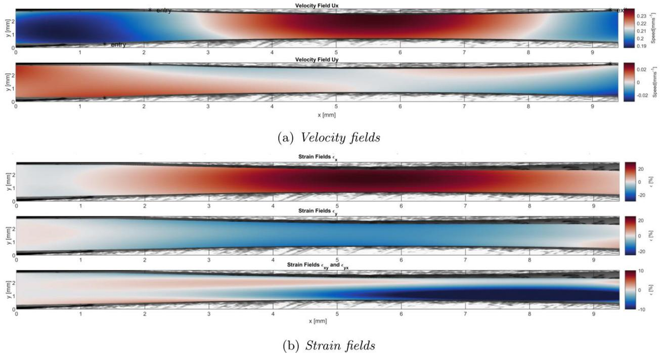
**Figure 1:** Robustly converged results for the Hand Mill case, with in (a) the velocity field in x and y direction and (b) the fields of the  $\epsilon_{xx}$ ,  $\epsilon_{yy}$ , and  $\epsilon_{xy}$  components of the Green-Lagrange strain tensor). Note that these results are preliminary as the analysis is still being further optimized.
