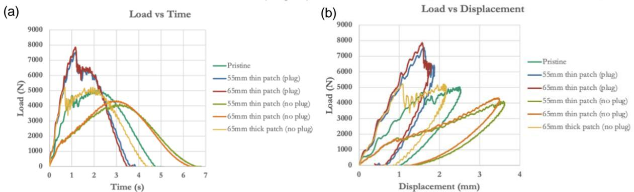
Figure 2: (a) Load vs time trace, and (b) load vs displacement trace for pristine, 55mm thin patch with plug, 65mm thin patch with plug, 55mm thin patch without plug, 65mm thin patch without plug and 65mm thick patch without plug repaired samples impacted at 7.5J
