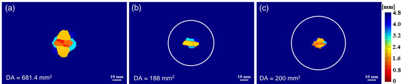
Figure 1. C-scan images after 7.5J impact of (a) pristine sample, (b) 55mm patch repair, and (c) 65mm patch repair
