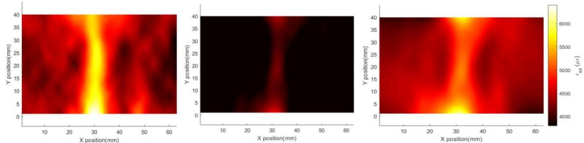
Fig. 2 Bending strains measured by DIC (left), predicted by a FE model using literature data (middle) and by an updated FE model (right).
