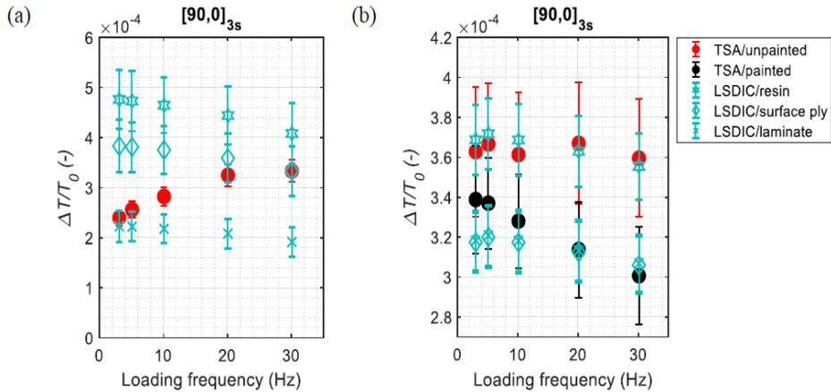
Figure 1.  $[90,0]_{3s}$  Normalised  $\Delta T/T_0$  vs Loading frequency of (a) CFRP and (b) GFRP [6].
