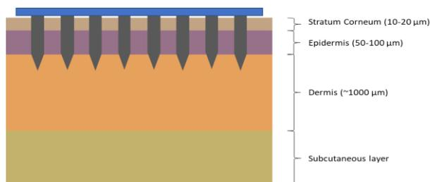
Fig. 1, Diagram of microneedles inserted into skin, penetrating to the dermis layer
