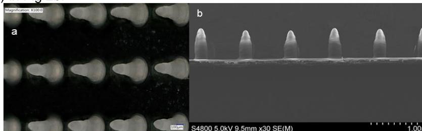
Fig. 2, showing SEM and 3D microscope images of the MSt arrays; 2a. 3D microscope image of the ML3DP solid MSts; 2b, SEM image of the ML3DP solid MSts
