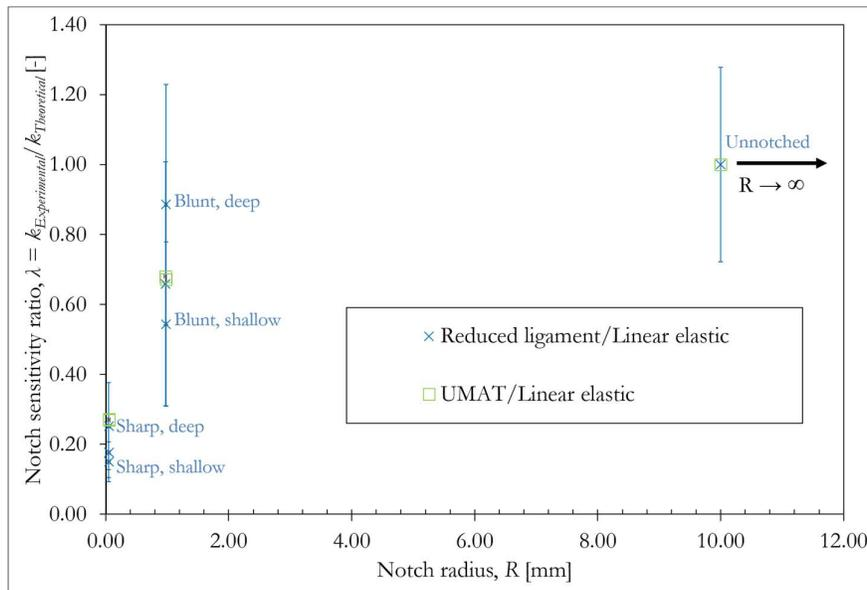
Figure 1: The dependence of notch sensitivity ratio on notch radius for the different geometries.
