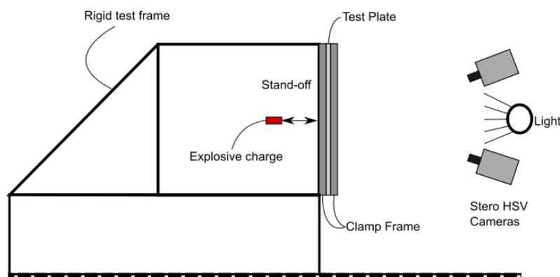
Figure 1: Experimental schematic showing the test plate, frame and camera setup.
