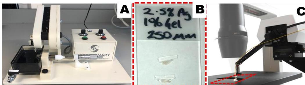
Fig. 1 Setup of the Compresstome® VF-210-0Z (a); PCTS 250µm thickness (b); set up of Optics 11 Chiaro Nanoindenter (c).
