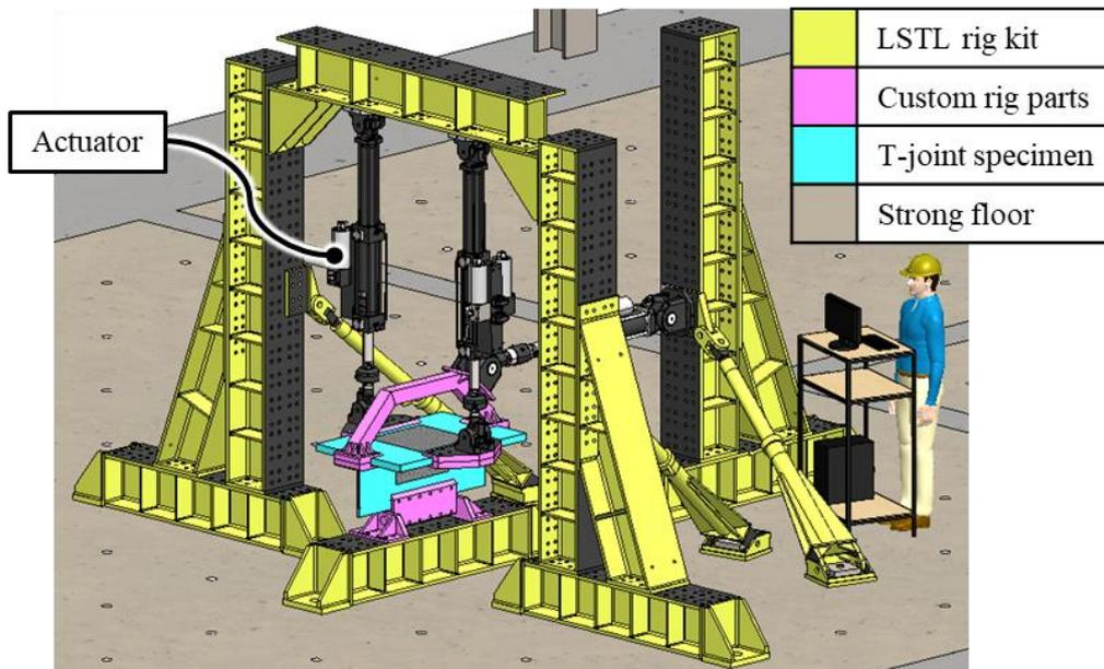
Figure 1: T-joint substructure multi-axial test rig in LSTL
