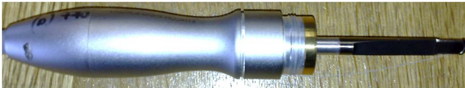
50kHz tuned ultrasonic cutting blade and handpiece
