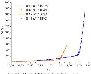
Figure 2 : PET and PEF true strain/stress curves obtained for the same equivalent strain rate of 0.1 s<sup>-1</sup>.
