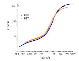
b) PEF and PET master curves at reference temperature temperatures of 100°C and 85°C respectively; E' is the elastic modulus, aT the shift factor and f the frequency.
