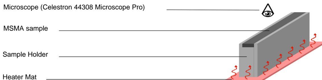
Fig. 1. Experimental setup
