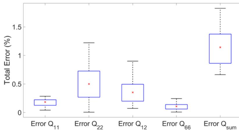
Figure 2 Total error (%) for a deep notch sample loaded at an angle. The mean value of each error is shown with a red 'x'. The edges of the box are the 25th and 75th percentiles. The minimum and maximum recorded values are shown with dashed lines.
